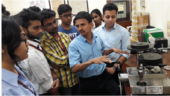
Demonstration of Dead Weight Tester inside the Pressure Calibration Laboratory
